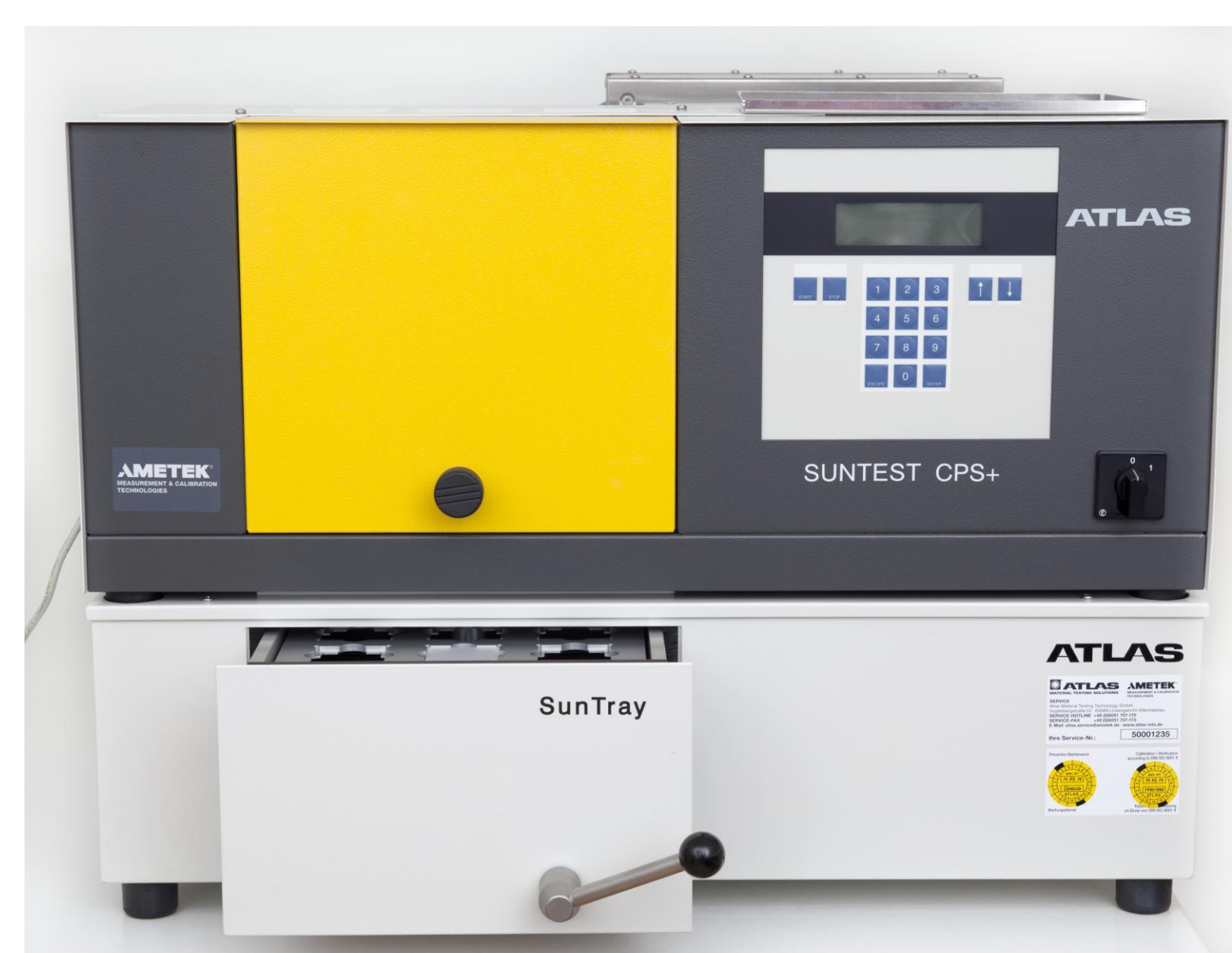
Figure 2: CPS suntest system – UV-source for irradiation.
